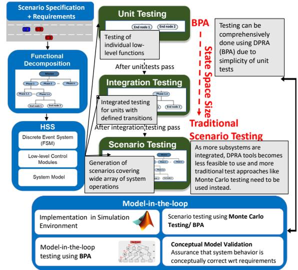
Fig. 1: Block Diagram of the Proposed Model-Based Testing Methodology
